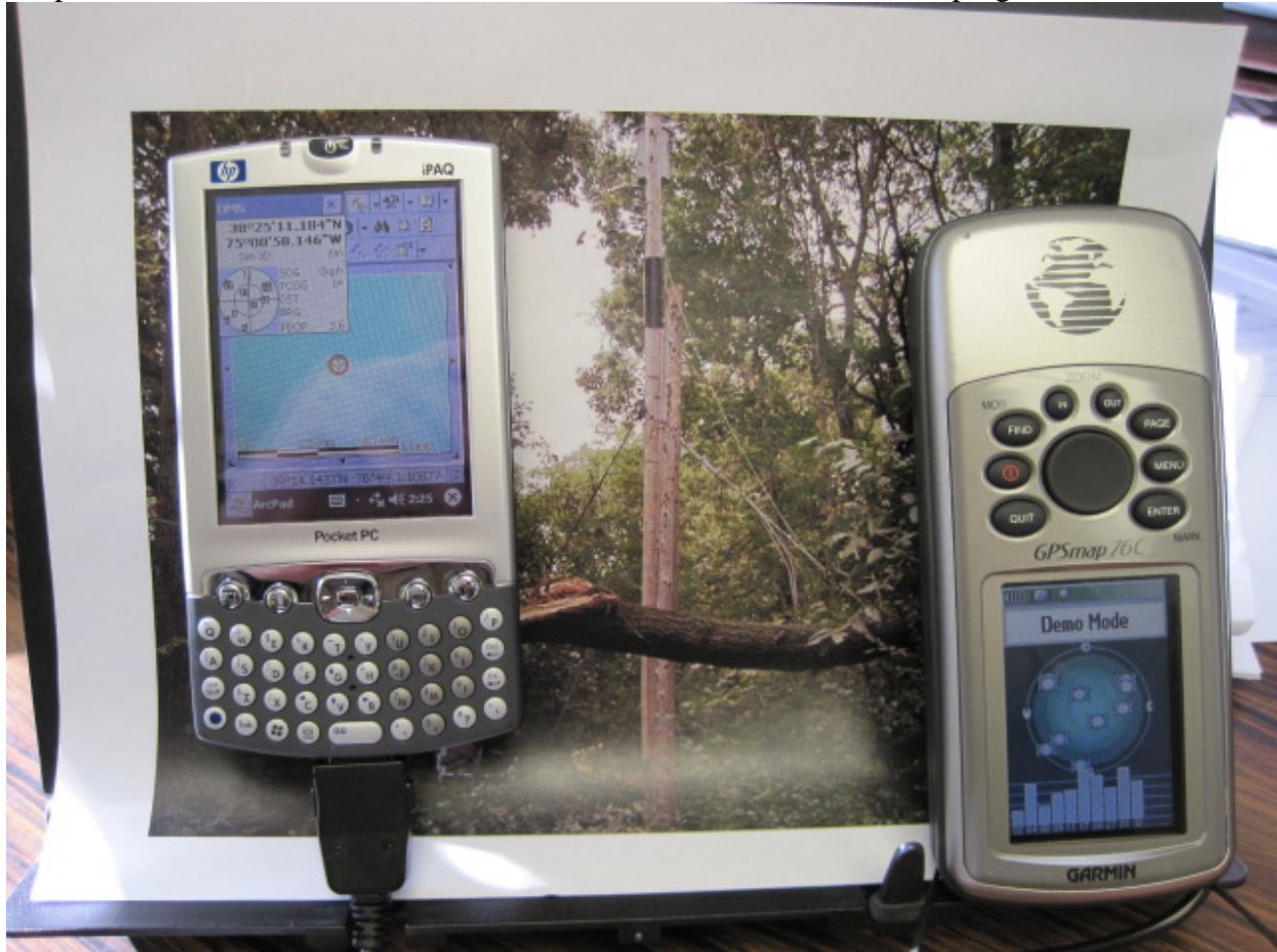
Figure 1. Pocket PC (left) showing ArcPad display screen with satellite window; positional data is received from GPS (right).
